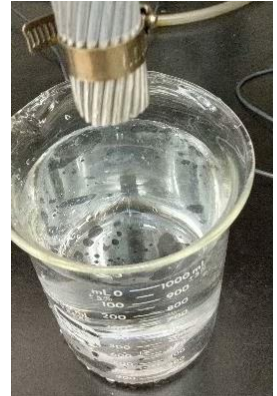
Video: when the superhydrophobic region is submerged in water there is a silvery sheen over the surface from an air film (processed surface remains dry even when submerged)
