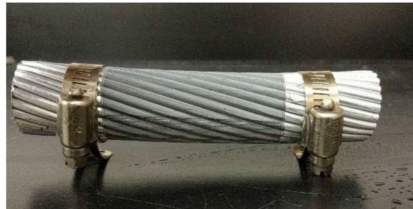
Video: note how the water droplets roll off of FLSP functionalized region and wick into the powerline on the unprocessed region
