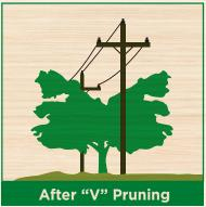
NOTE: The illustrations above show how trees growing too close to power lines can be trimmed to protect tree health while providing necessary line clearance for reliability and safety.
